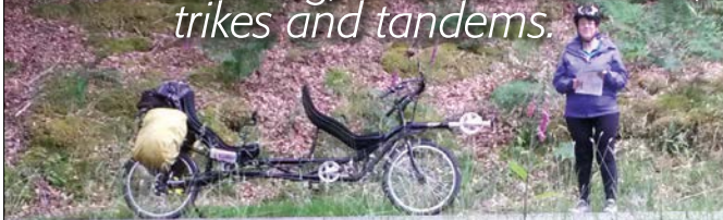
Nazca Quetzal folding recumbent tandem - folds to less than length of standard bike / fits train bike space
